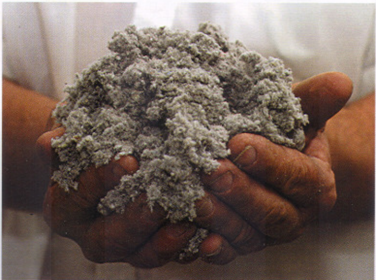
Eco Insulation is made out of recycled newspaper - good for the environment and those who use it
